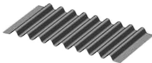
Fig. 4 The CAD model of the corrugation type PEN prototype
