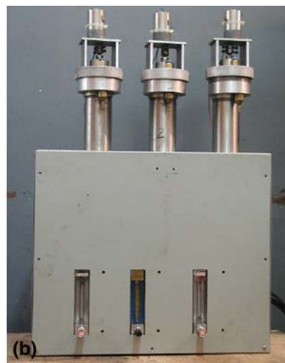
Fig. 1 The principle sketch (a) and photograph (b) of the three-hopper powder feed device
